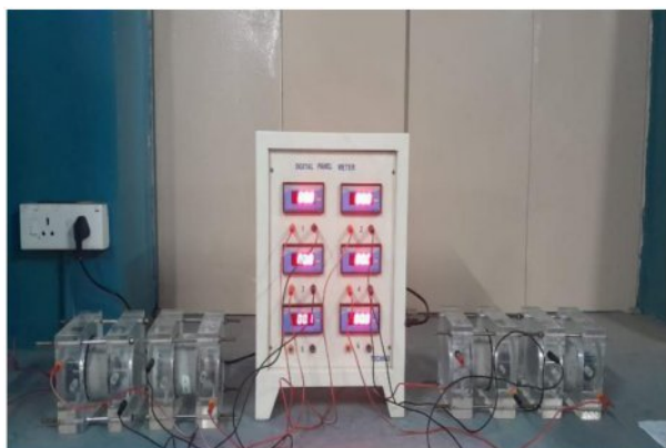
Fig. 3. Rapid Chloride Penetration test.
