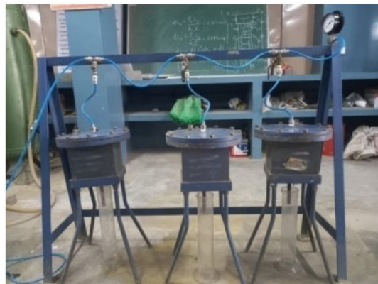
Fig. 4. Water Permeability test.
