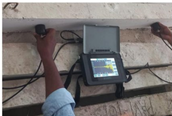
Fig. 25. Ultrasonic Pulse Velocity Test.
