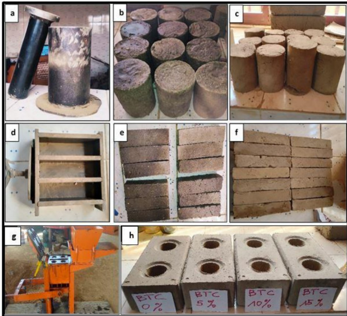
Fig. 4. Preparation of adobes for the different tests: (a) Molds of cylindrical samples (b) Superior view of the cylindrical adobe samples (15.5 × 8 cm); (c) Molded cylindrical samples; (d) Prismatic molds; (e) Superior view of the prismatic adobe bricks (15.5 × 4 × 3 cm 3 ); (f) Molded prismatic samples; (g) Manual press for compressed earth bricks; (h) Superior view of the adobe bricks made using manual press (29.5 × 14 × 8 cm 3 ).
