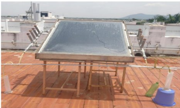
Fig. 2. Modified Solar Still (MSS).
