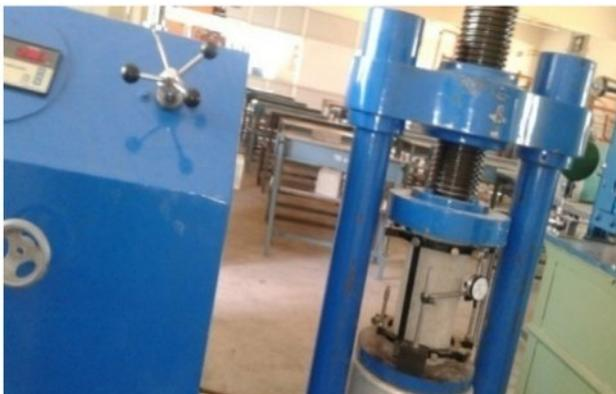
**Fig. 1.** Modulus of Elasticity Specimen Test Setup.
