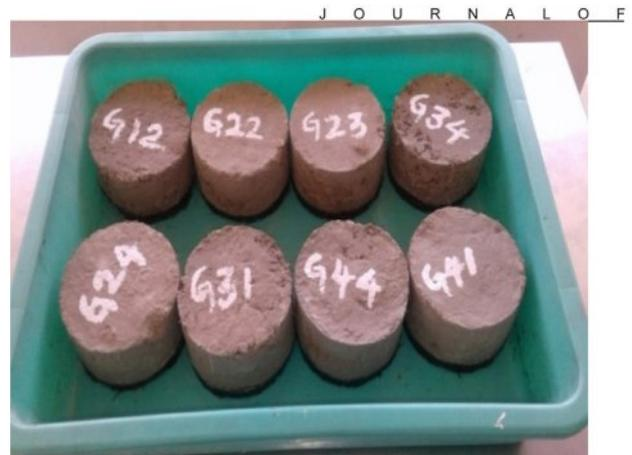
**Fig. 2.** Testing of Concrete Specimens for water absorption in Capillarity.
