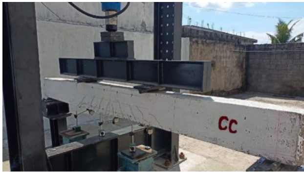
Fig. 1. Crack Pattern and Failure Mode of CC Specimen.
