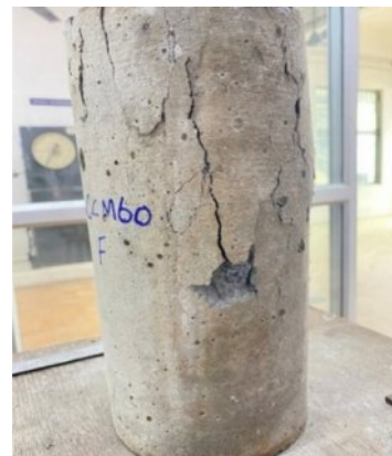
Fig. 5. Failure of Specimens due to Modulus of Elasticity test.
