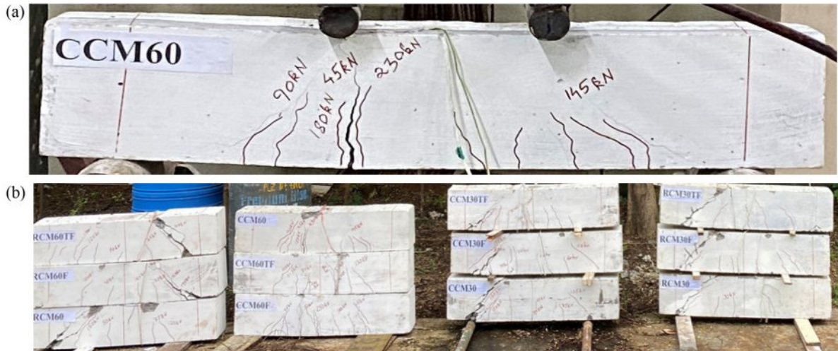
Fig. 7. a) Failure of Conventional Beam under Flexural Testing b) Failure of all Beams Under Flexural Testing.
