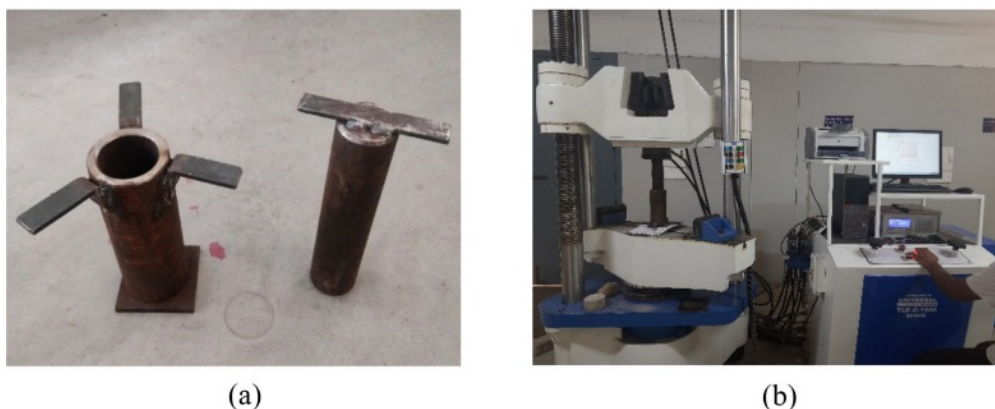
Fig. 3. Representation of (a) Mould and Shaft and (b) Controlled universal testing machine.
