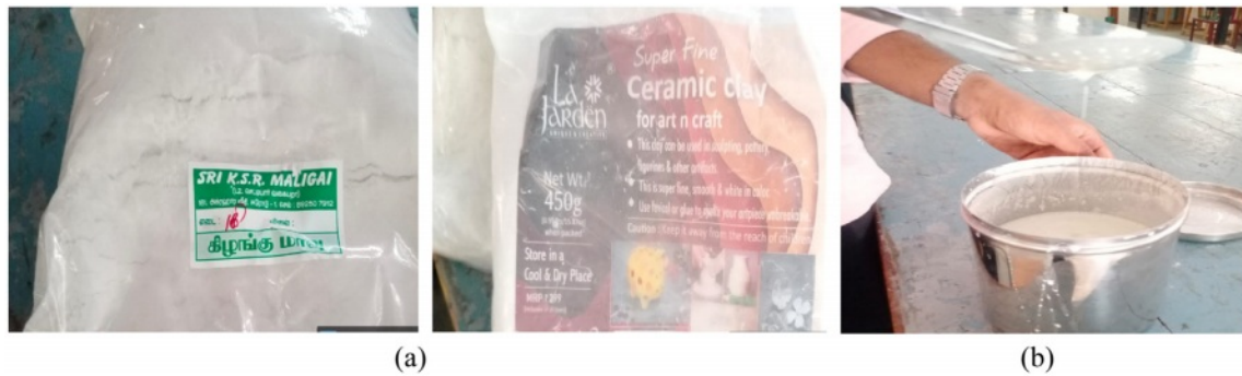
Fig. 2. (a) Cassava starch and Ceramic powder, (b) Combined Binder.
