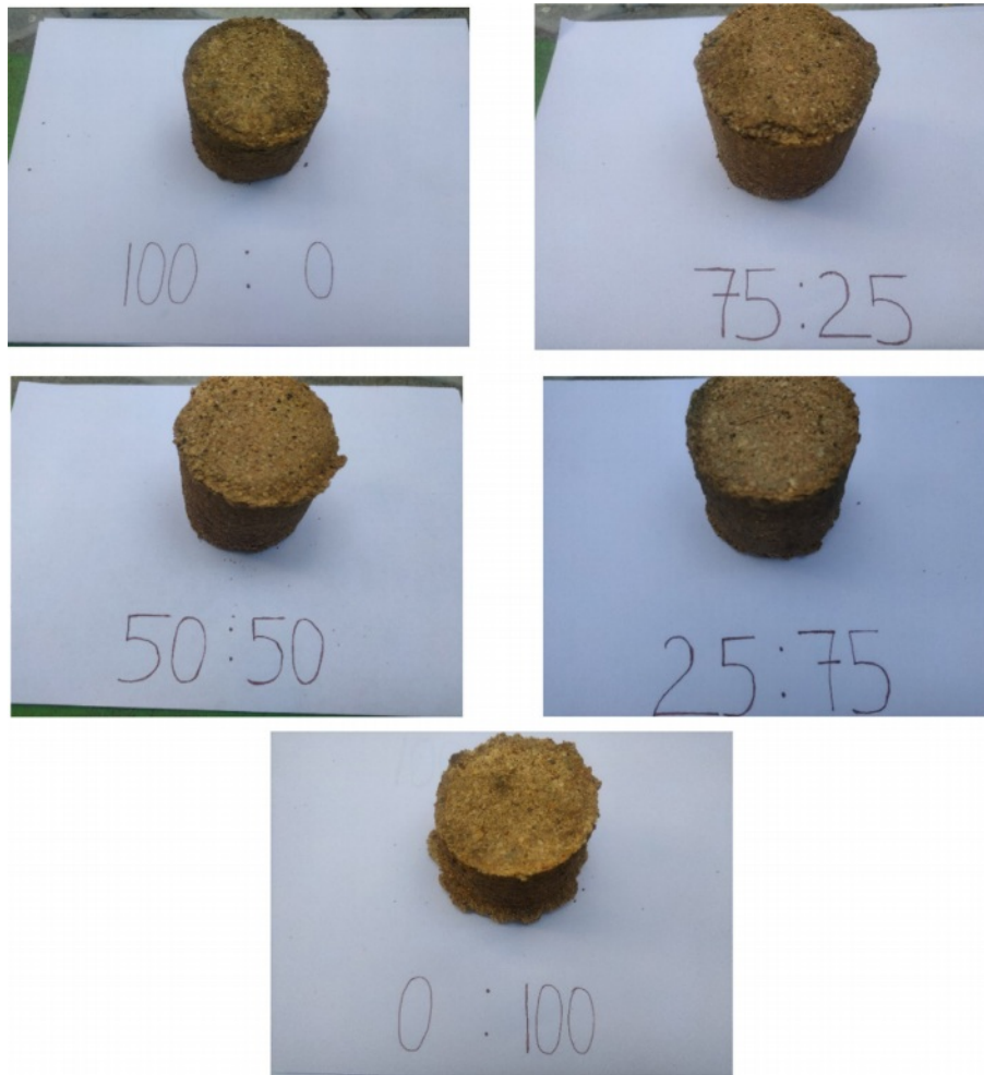
Fig. 4. Briquette samples of various proportions.
