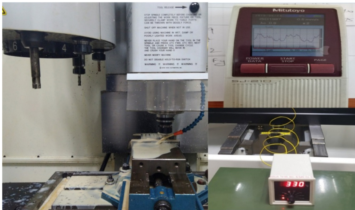
Fig. 5. Experimental Setup with temperature and surface measurement.
