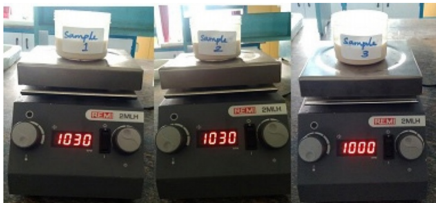
Fig. 2. Preparation of Cutting fluid by stirrer.
