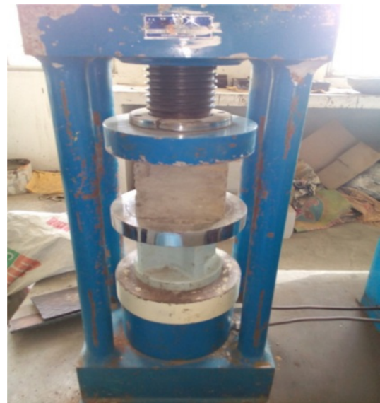
Fig. 1. Compressive strength test.
