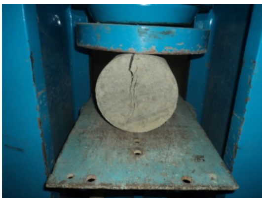
Fig. 2. Split tensile strength test.
