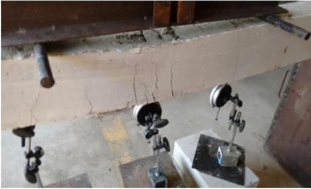
Fig. 4. Beam specimen under static load test.
