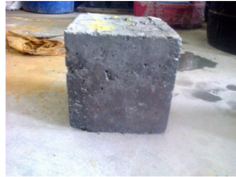
Fig. 6. Typical surface of the cube after 90days of sulphate attack.
