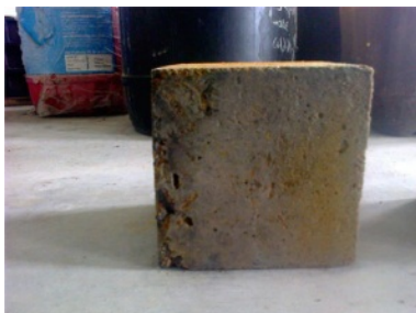
Fig. 5. Typical surface of the cube after 90days of acid attack.
