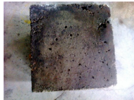
Fig. 7. Typical surface of cube after 90days of chloride attack.
