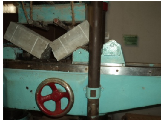
Fig. 3. Modulus of rupture strength test.
