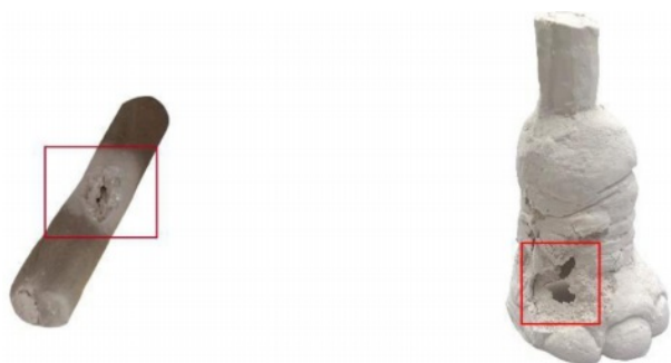
Fig. 3. Damage due to model breakage Cy_2 and Be_4 from left to right.
