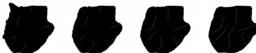
(b) Expansion of internal microcracks in recycled aggregates arising from particle shaping
