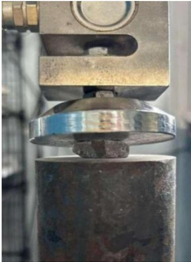
Fig. 4. Experimental setup for the property of recycled aggregate particles.
