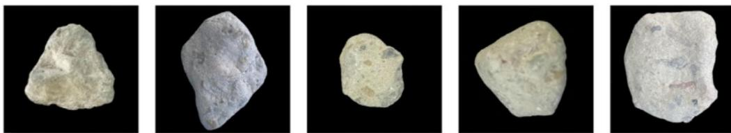
(a) Recycled aggregate particle morphologies with varying particle shaping time
