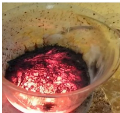
Fig. 2. Combustion reaction of reactant producing LiZnCu ferrite.
