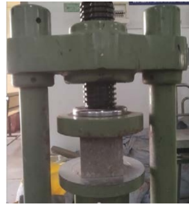
Fig. 2. ECC compression strength test setup.
