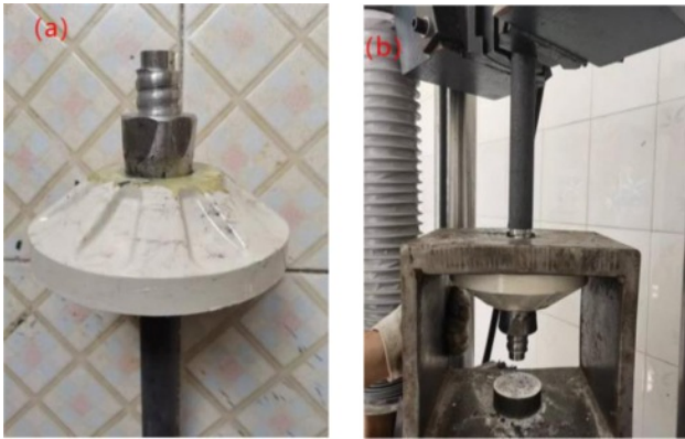
Fig. 10. bearing test (a) composite tray with metal bolt and nut (b) test condition.
