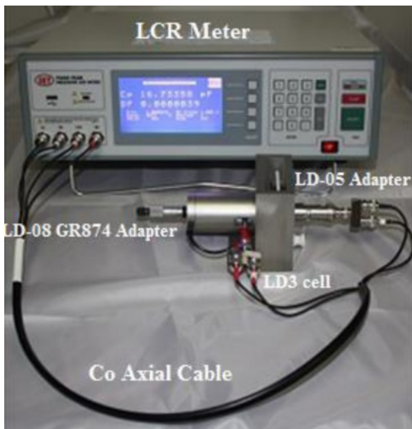
Fig. 10. Experimental setup of dielectric constant and dissipation factor.
