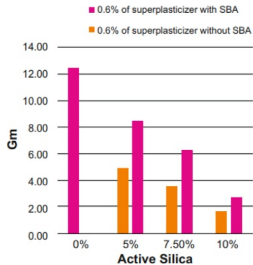
Fig. 7. Behavior of mortars with 0.6% of chemical additive regarding additions of silica fume with and without SBA in its composition for the Gm index.
