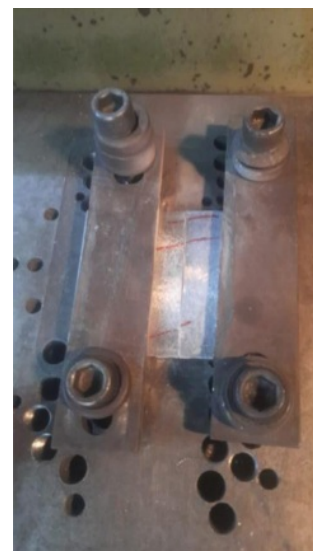
Fig. 3. Fixture to hold the workpieces.
