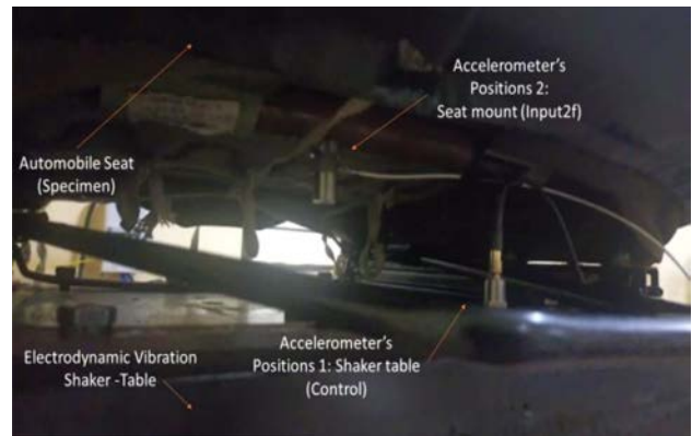
Fig. 2. Automobile Seat Mounting and Accelerometer sensor.
