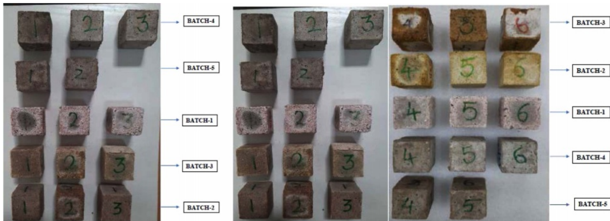
Fig. 5. Appearance of specimens after acid attack.
