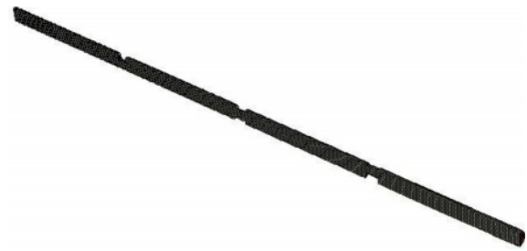
Fig. 4. Symmetrical half cylinder tube with orifice type blockages and 60% BR meshed in a semi-structured mesh.
