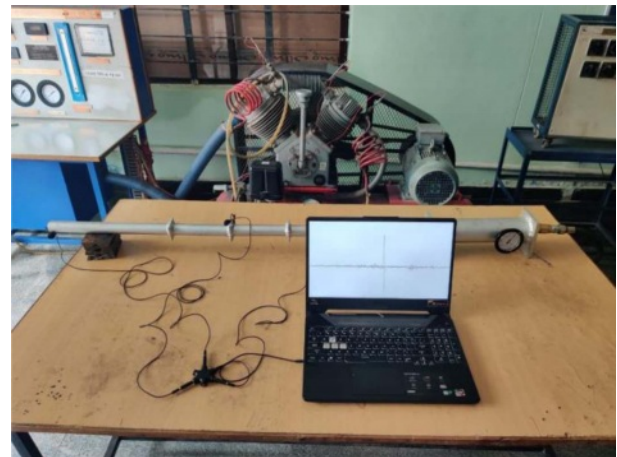
Fig. 7. Experimental setup for cylindrical cross section mounted with 13 layers of aluminium diaphragm.
