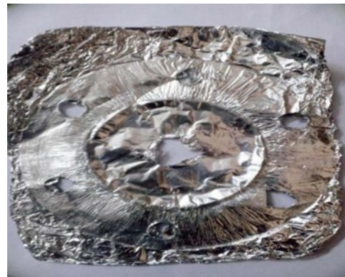
Fig. 13. 13 Layers of Aluminum foil blasted at 6.213bar Gauge Pressure.
