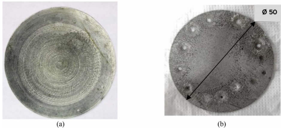
Fig. 5. Workpiece [Anode] (a) Before machining, (b) After machining.
