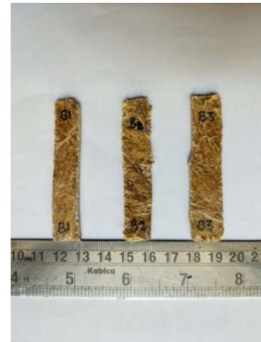
Fig. 4. Impact test specimens after fracture.
