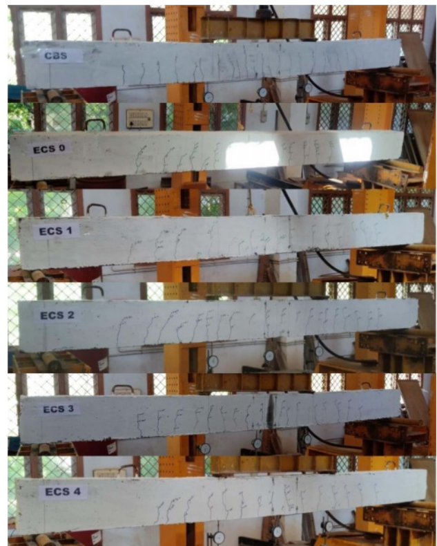
Fig. 4. Crack Patterns of Beams.
