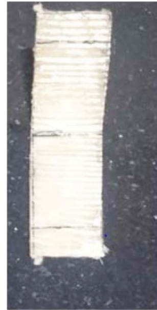
Fig. 8. Failure of the specimen after tensile testing.
