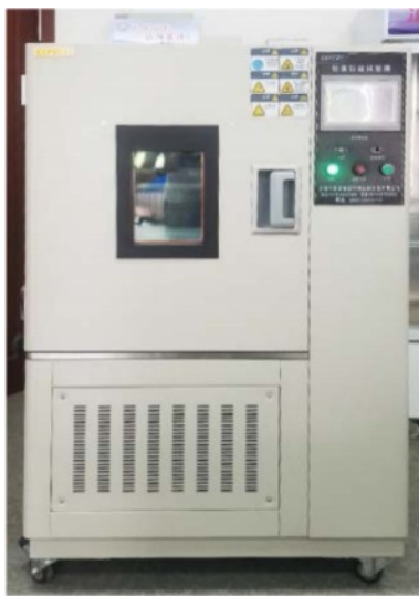
Fig. 3. Constant temperature and humidity curing box.
