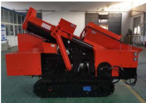
Fig. 1. Tidal concrete shotcrete unit.
