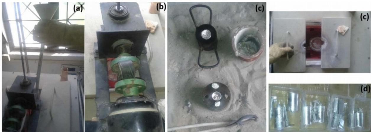
**Fig. 3.** Stir casting set-up. (a) Electric furnace with hopper to add powder. (b) Stirrer assembly for 90° axis change. (c) Casting tray and molds, with cast composite ingots. (d) Furnace muffle. (e) Cast ingots.
