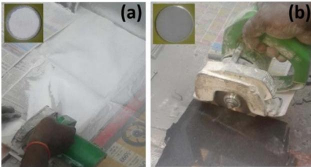
**Fig. 2.** Marble (a) and Granite (b) dust powders obtained from the construction site.
