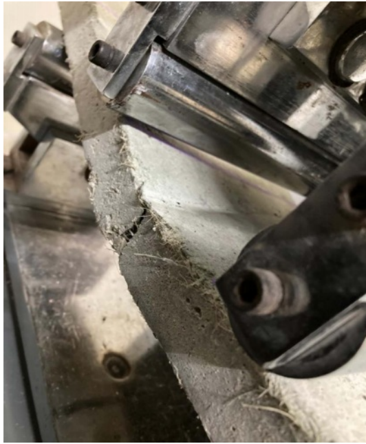
Fig. 7. Testing of shear specimen in CTM.
