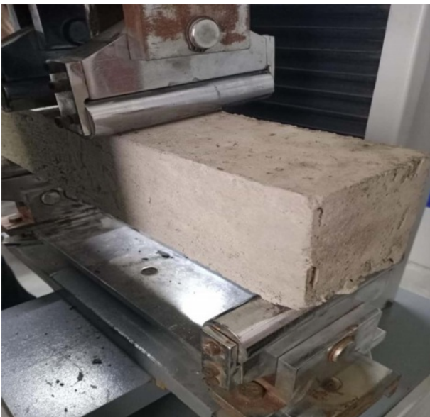
Fig. 4. Loading of beam specimen.
