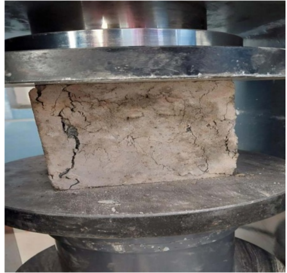
Fig. 5. Propagation of crack under the roller.
