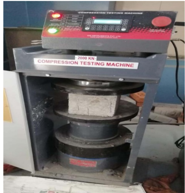
Fig. 2. Testing of concrete cube specimen in CTM.
