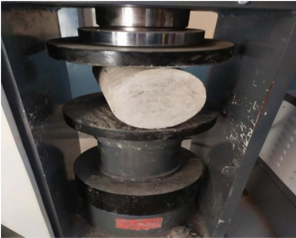
Fig. 3. Testing of cylinder specimen in CTM.
