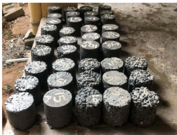
Fig. 7. Cured permeability cylinders.
