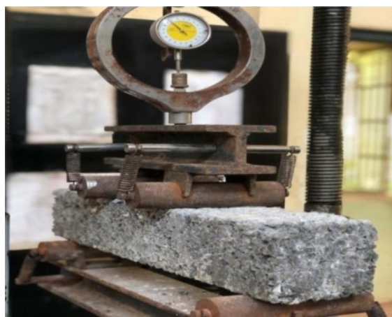
Fig. 6. Flexure test on PC.
