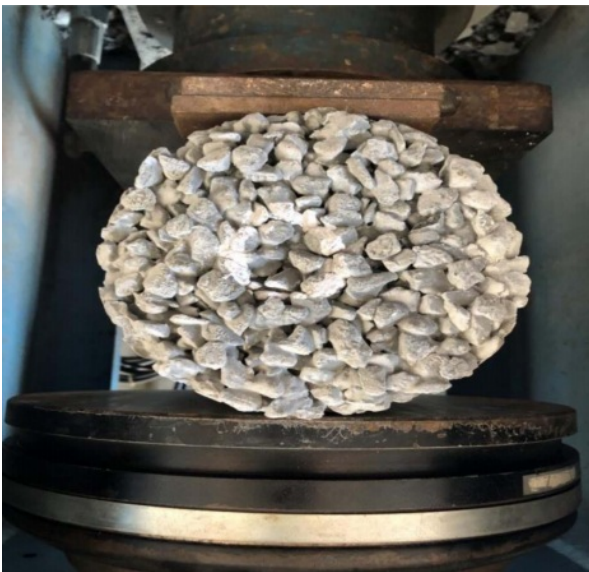
Fig. 5. Split tensile test on specimen.
