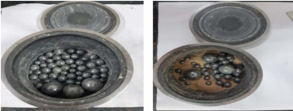
Fig. 5. Ball milling cylinder and balls.
