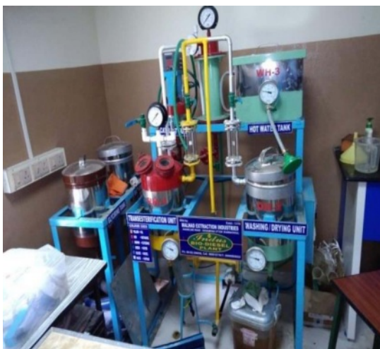
Fig. 3. Biodiesel Transesterification Plant.
