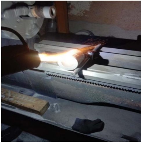
Fig. 5. WC Thermal Barrier Coating.
