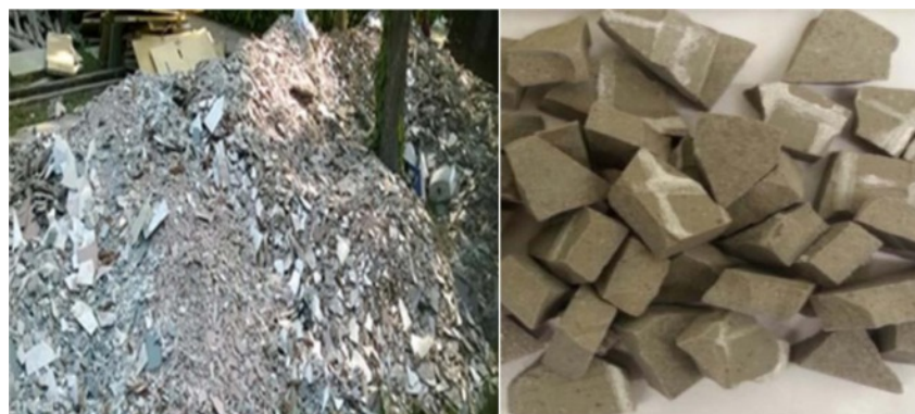
Fig. 3. (a) Demolition of ceramic wall tiles [12]. (b) Ceramic tile waste –4.75 to 20 mm [70].
