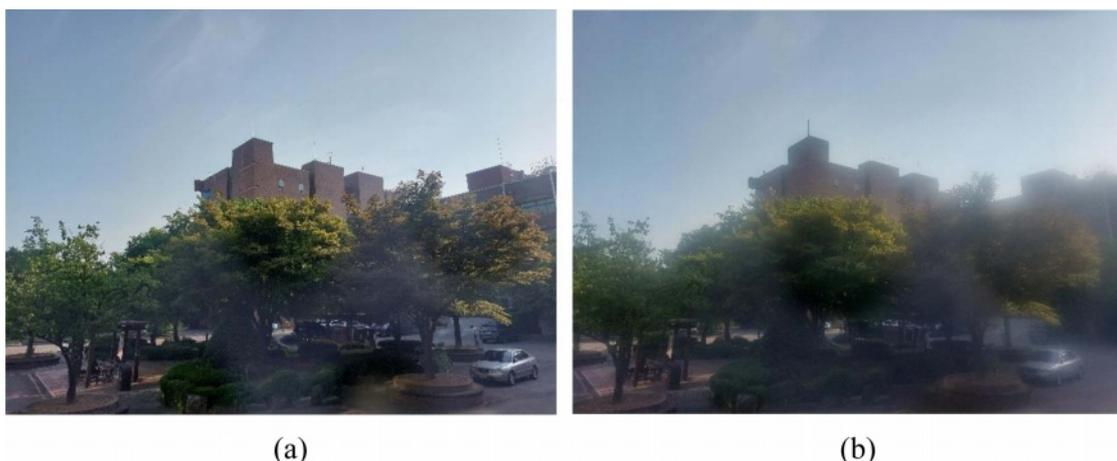
**Fig. 6.** View of the building observed through the B-series glass. (a) HF 10% (haze = 6.8%), (b) HF 15% (haze = 9.9%).
