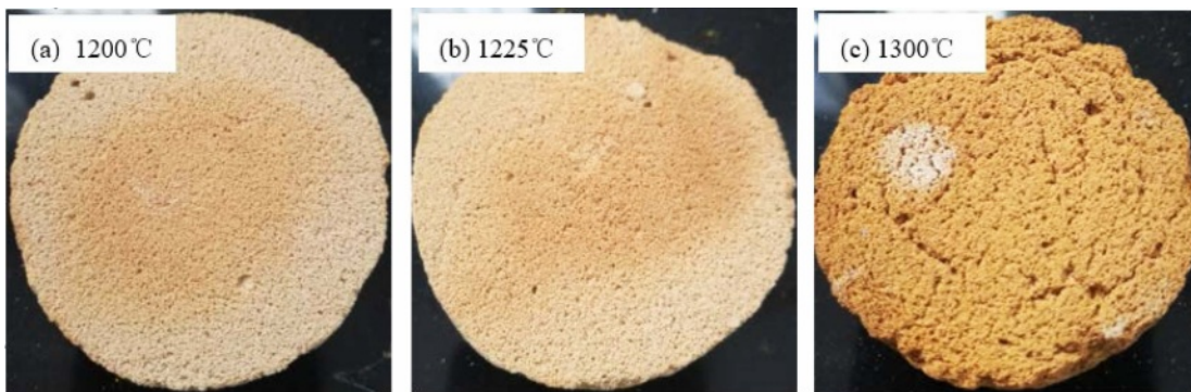
Fig. 4. Surface morphologies of permeable bricks prepared at different sintering temperatures.
