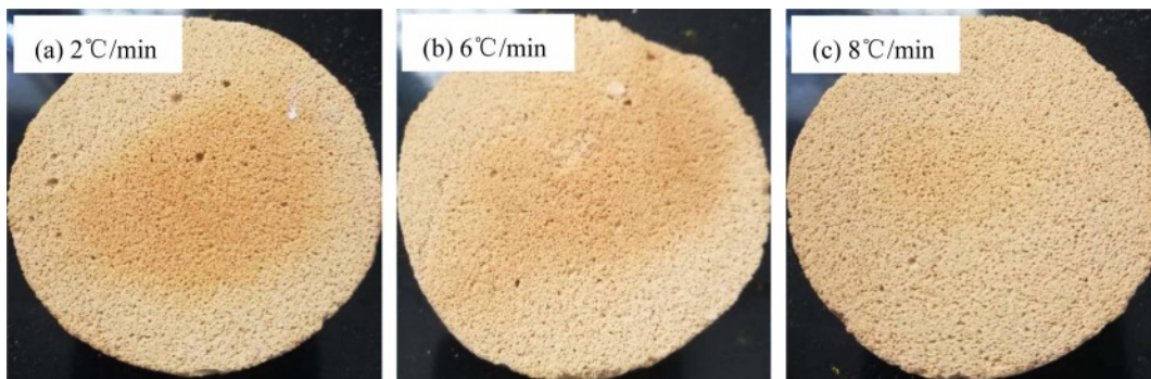
Fig. 10. Microstructures of permeable bricks prepared at different heating rates.
