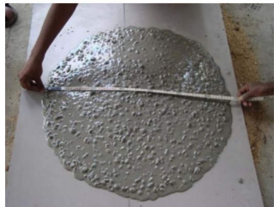
Fig. 2. Slump flow test.
