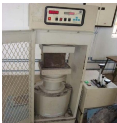
Fig. 1. Compressive test on cube.
