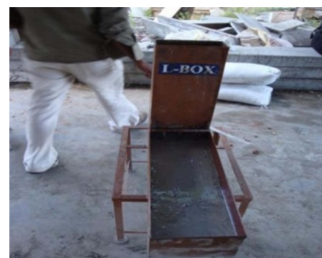
Fig. 3. L box test.
