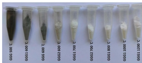
Fig. 4. The pictures of GGG, GGG1, and GGG2 nanopowders annealed from 500 to 1200 °C.
