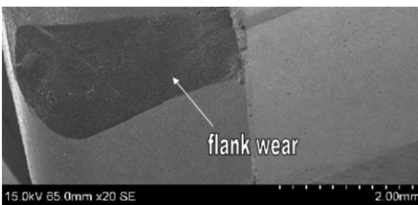
Fig.7 (a). SEM/Insert at V=70m/min, S=0.15mm/rev, ap=0.80mm
