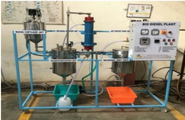
Fig. 1. Transesterification Biodiesel plant.
