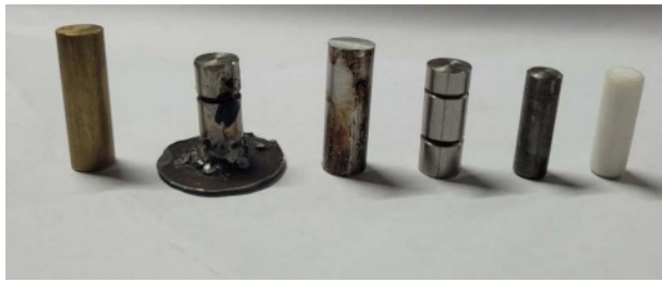
Fig. 2. Specimens -brass, titanium, mild steel, stainless steel, aluminum and teflon.
