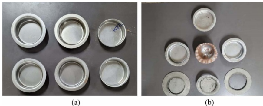
Fig. 4. (a) Drawn Product and (b) Defective Product.
