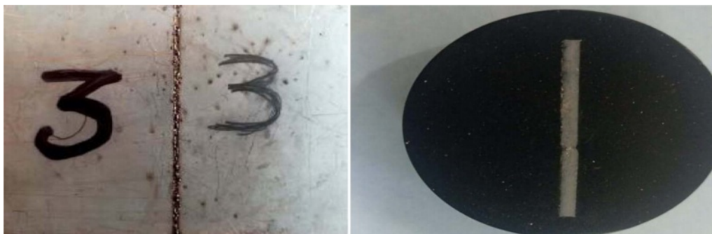
Fig. 2. Dissimilar material welded by laser beam welding
