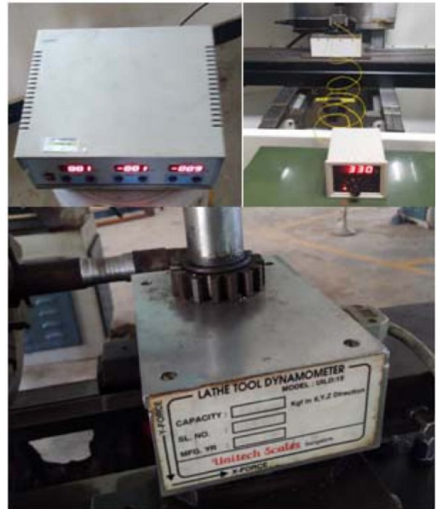
Fig. 5. Experimental setup – Lathe Tool Dynamometer, Thermocouple arrangement.
