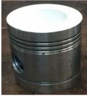
Fig. 5. Mullite – 10% \text{La}_2\text{O}_3 – top coat and NiCr bond coated piston.
