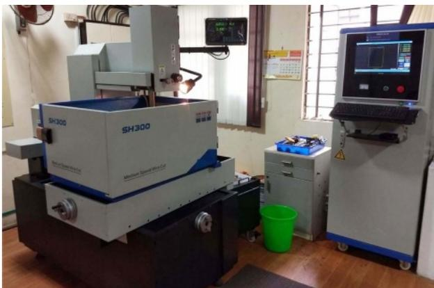
Fig. 3. Photographic view of Reciprocated travelling WEDM.
