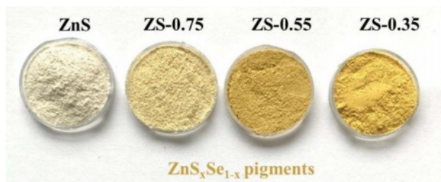
Fig. 6. As-synthesized ZnS_xSe_{1-x} pigments.
