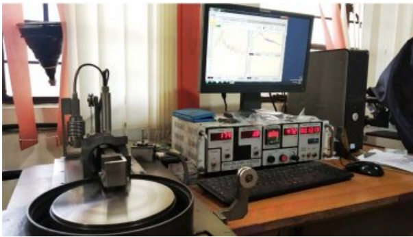
Fig. 4. Experimental setup for wear test.
