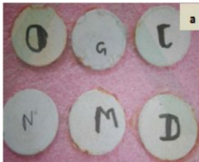
Fig. 4. ML and MZ Test specimens after salt spray test for 100 hrs (O as MZ1, G as MZ2, C as MZ3 and N as ML1, M as ML2 and D as ML3 coatings).
