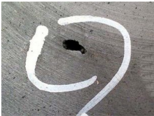
Fig. 7. Sand inclusions defect.
