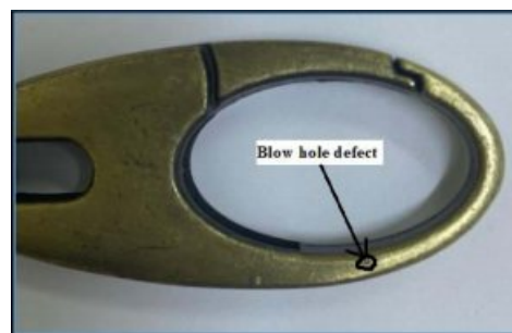
Fig. 2. Blow hole defect.
