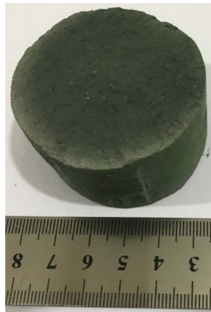
Fig. 7. Oxidation behavior of the optimum specimen (t-zirconia: 3.267 wt.%, MgO: 4.101 wt.% and fine-grained graphite).
