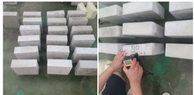
Fig. 3. Mortar samples with shielding materials.
