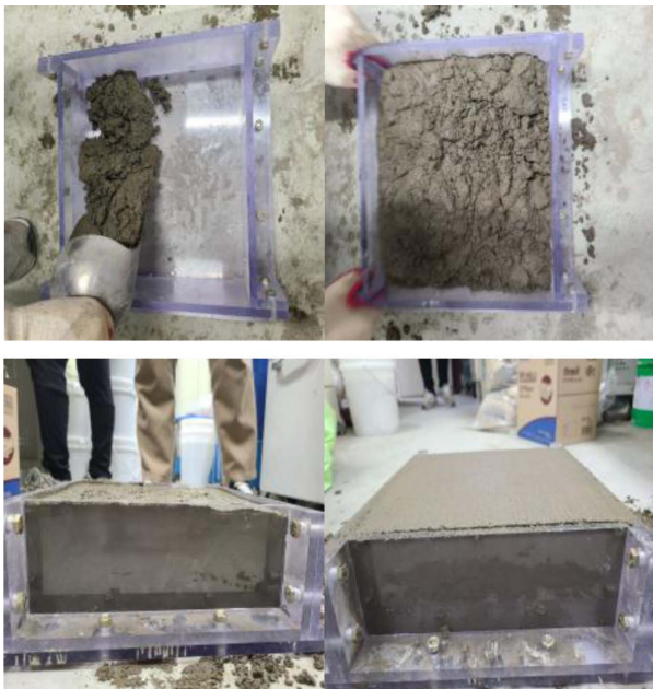
Fig. 2. The process of preparing the mortar sample.
