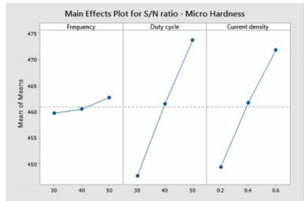
Fig. 3. Mean S/N ratio for Micro Hardness.
