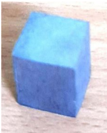
Fig. 12. Coated specimen after corrosion test
